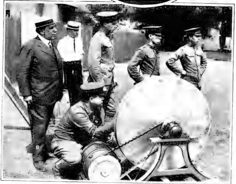
The Gun Consists of a Wheel Constructed of Aluminum and Copper Mounted on a Frame and Rotated at High Speed by a Motor
